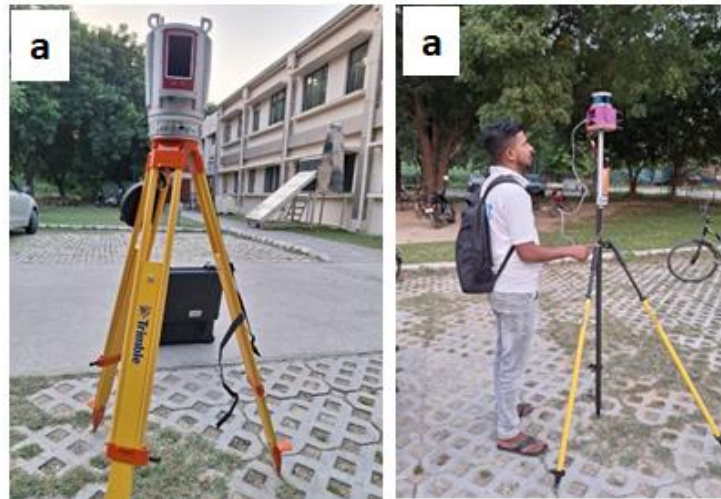
Fig. 1 Experimental setup for (a) RIEGL VZ-2000 and (b) Velodyne VLP16.
